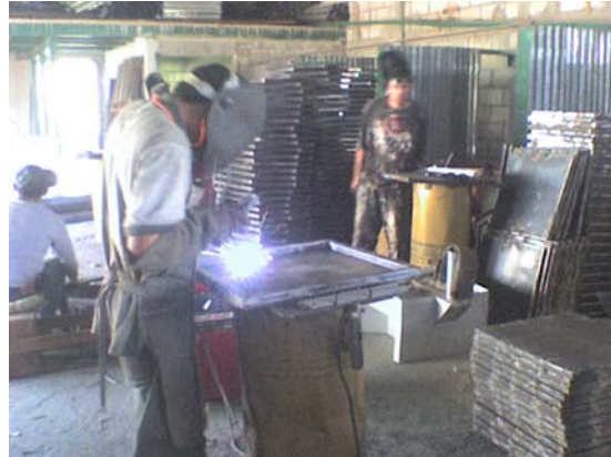
Assembling and welding the pieces
