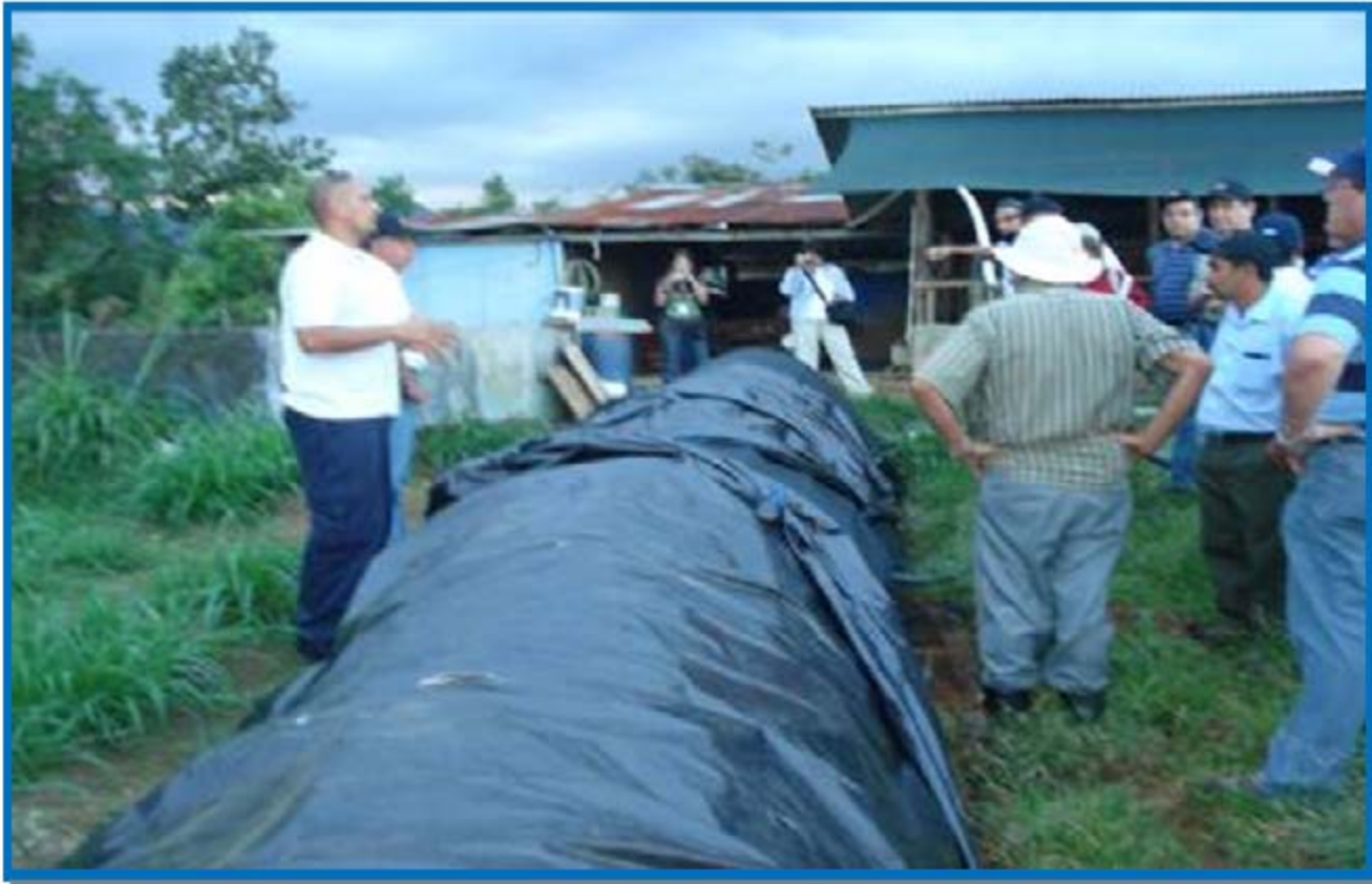
Bio-digester, located at the area of influence of Hydroelectric Project Peñas Blancas, owned by a local farmer. This practice avoids the cut of wood for cooking purposes.
