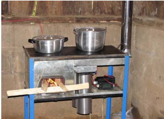
Detail of the stove unit; assembly of the eco-stoves
