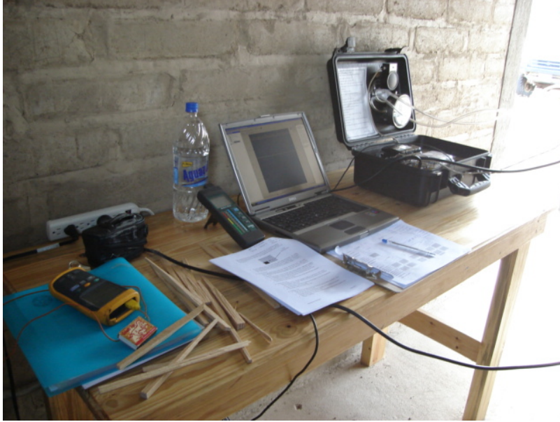
Photo 4: Portable Emission Measurement System (PEMS) installed in the Certification Center.
